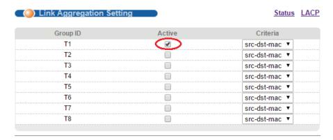
Below, set the ports you will use to link aggregate as T1. In this case, the core switch is currently physically connected to port 20. A second and third cable will be attached on port 21 and 22 afterwards.
