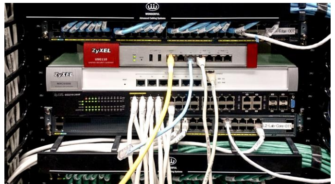
Image 2: Zyxel gateway, WLAN controller, L2 PoE switch were used during the event (from top to down)
